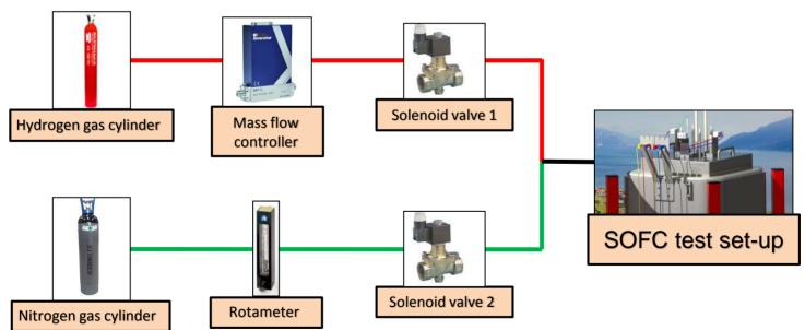
When hydrogen is detected by the detector, valve 1 (hydrogen) is shut down and valve 2 is opened, purging the system with nitrogen, preventing further release of hydrogen.
