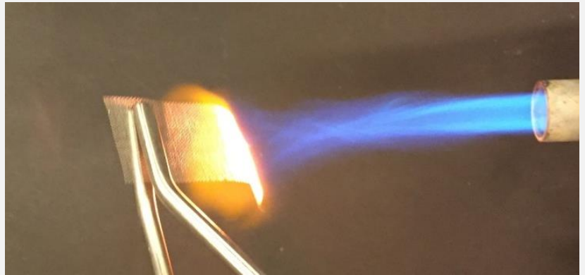
With elevated melting point (1768 °C), platinum M_Grid™ can be used with SOFC at high temperature (>900°C) and long periods of time (>100h)
