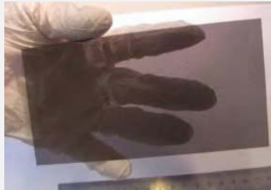
Crofer 22H M_Grid™ coated with 5-10 \mu m of CuMn_2O_4 for interconnect improvement.
