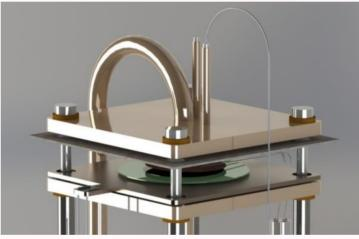
Open Flanges head with fuel diffuser and double thermocouple holder for optimal cell temperature control
