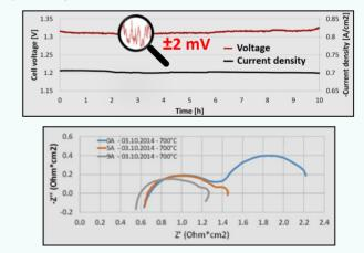
Electrolysis test done at EPFL (JVH group, Swiss Institute of Technology, Lausanne) with the integrated steamer, and impedance spectroscopy on the cell during electrolysis mode.
