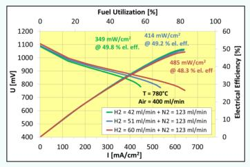
Test conditions: Open Flanges<sup>TM</sup> Set-Up with a 2R-Cell (cathode SA:  $10.2 \text{ cm}^2$ )
