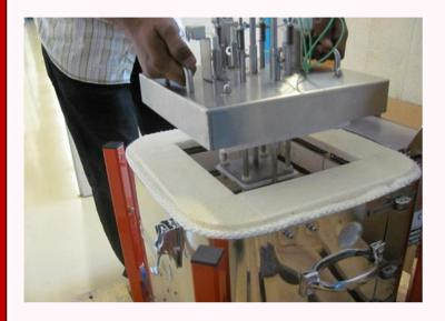
End of broken cells and secure testing: the cell is squeezed by a soft alumina felt that prevents any damages, the excess fuel burns continuously in the alumina felt at the cell edges
