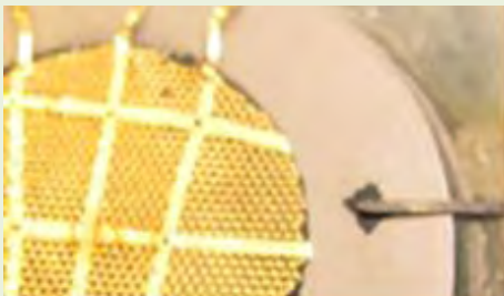
2R-Cell™ after a test and redox cycles in the Open Flanges Set-Up. Gold grid is used to collect current on cathode side
