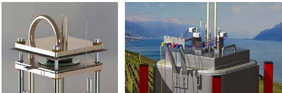
Figure 2. Left : Exploded view of the set up head. Right : Drawing of the Open Flanges™ Set-Up developed by Fiaxell in a furnace.
